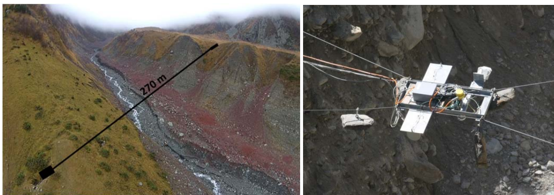
Figure 3.9: Location A (left) where gauge radars for the alarm system will be positioned on wire ropes (right).
