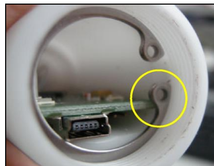
Figure 2: The retaining ring prevents the print from pulling out and being damaged. It has to be in a position as shown by the yellow circle.
