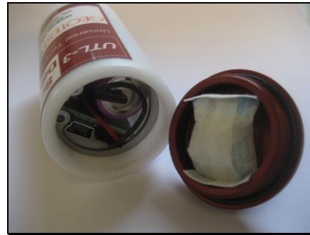
Figure 4: Before closing UTL-3 Scientific Datalogger, put a silicagel minibag back into the cap.
