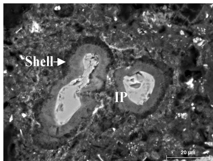
Figure 16: Aventicum mortar, morphology of the cement grains (original quartz core and C_2S rim) showing inner and outer hydration products discriminated by a hollow shell.
