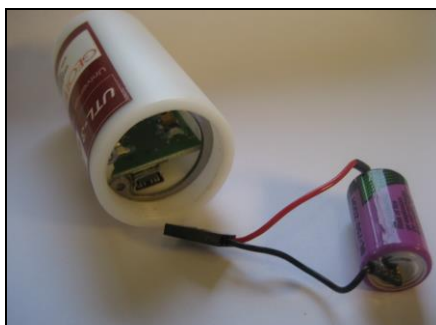
Figure 1: Pull out the battery carefully and unplug the black socket.
