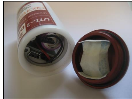
Figure 4: Before closing UTL-3 Scientific Datalogger, put a silicagel minibag back into the cap.
