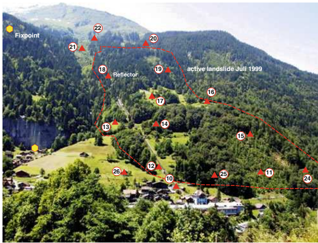
Fig. 3 Landslide of Gryfenbach as an example of a continuous landslide with indication of boundaries and tachymetric measuring points. Without the tachymetric dataset velocities can hardly be defined
