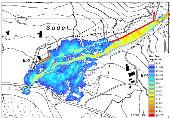
Figure 1. Debris flow modelling at Sädelgraben in Schangnau with RAMMS using NoFlux-cells for protection dams (red and orange lines).
